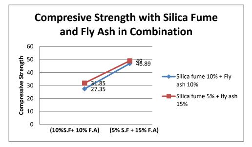
M40 grade concrete compressive strength incorporated with combination of silica fume and fly ash as replacement under HCL attack:
