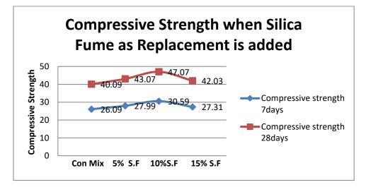
M40 grade concrete compressive strength incorporated with combination of silica fume and fly ash as replacement:
